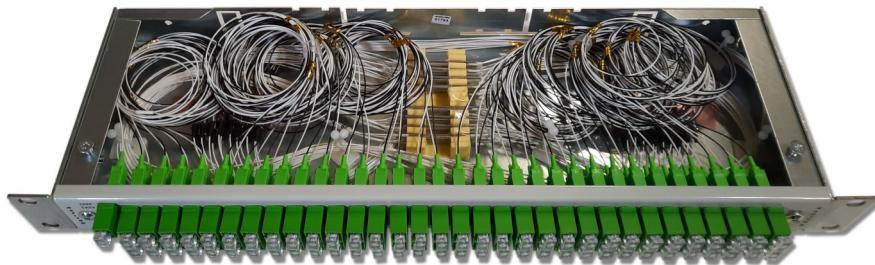
The picture above shows a 19" panel with 32 PON-WDMs with 1550 nm port spliced on a 1:32 splitter. The connectors are SC/APC. Technical information about PON-WDM and OADM can be found in the [Specs section of the product catalog](#).
