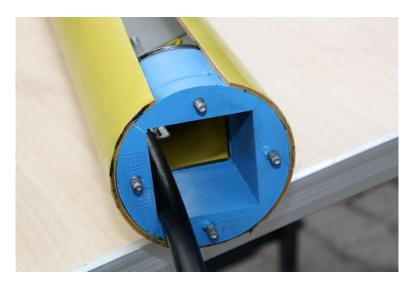
Push pass-through frames to the ends of the tube.
