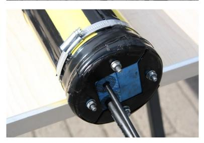
Finally, tighten the nuts of the pass-through frames at the ends of the joint closure. Tightening should be done carefully to ensure that the pass-throughs are properly sealed.
