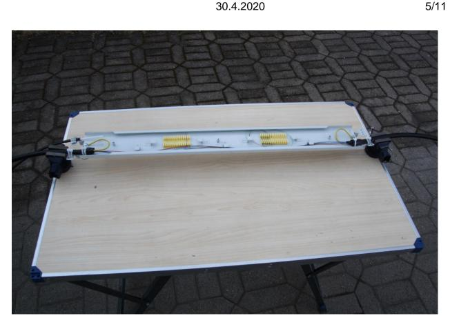
The cables have been attached to the splice tray and the branched fibers have been spliced. Finally, to protect the fibers, secure the plexiglass cover that comes with the splice tray.
