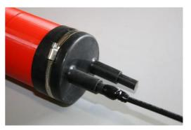
Cable gland sealed with PVC-surfaced vulcanized tape.
