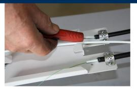
Cut the central tubes of the cables with a tool for this purpose.
