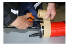
The tape is rotated with the protective paper a turn around the housing, leaving a small overlap and cutting the required length.
