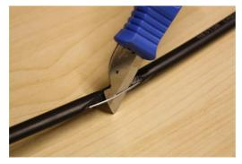
Carve out the steel elements at the marked point for 30 to 50 mm in length.
