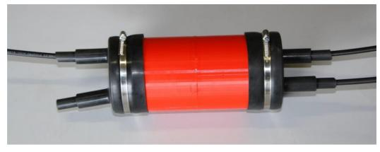
Lock the end pieces to the frame tube with the hose clamps that come with the joint closure. When installing the hose clamps, note that they are straight and between the raised stripes at the ends of the frame tube!
