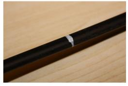
Mark the place for grounding to one of the cables coming into the joint closure with steel traction elements.
