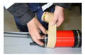
Finally, the tightness of the frame tube and end piece seam is ensured with a layer of vulcanizing tape.
