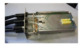
The shrinkage is done and the fibers are waiting to be spliced.
