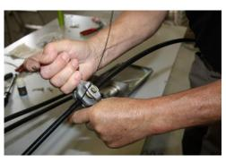
You can split the sheath and the corrugated steel plate underneath the sheat with ST-OCS splitting tool. In this case, with the blade of the splitting tool, the sheating is split from the grooves of the steel wires. This should be done on each side.
