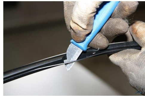
Dig out the steel wires.
