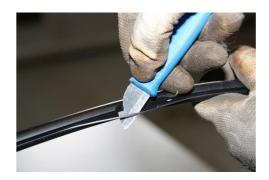
Dig out the steel wires.
