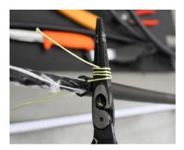
Turn the tear wire around a screwdriver or pliers and pull the wires to make the sheath break.
