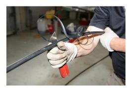
Peel the sheath off the steel wires along the entire length to be peeled.
