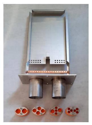
The inner part of the joint closure and the fitting mechanical cable glands for different cable diameters. Starting from the left: 2x20mm (7263240), 4x15mm (7263241), 2x15mm+3x10mm (7263242) and 6x10mm (7263243)
