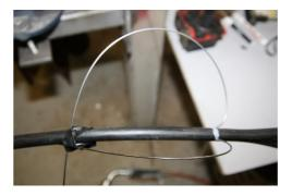
Bend the steel wires backwards and lock them with e.g. insulation tape to prevent damage from their sharp ends.
