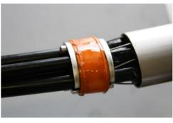
Push the cable gland with cables inside the oval pass-through at a depth of 5 to 15 mm and tighten the screws until the cable gland remains in place.
