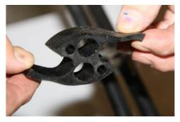
Split the sealing piece of the cable gland with a sharp knife
