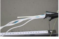
Cut any filling elements at the peeling point and leave the middle element to about 10 cm in length.
