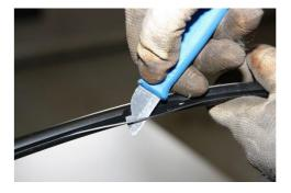
Dig out the steel wires.
