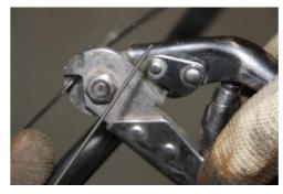
Cut the steel wires at each end to a length of about 20 cm.
