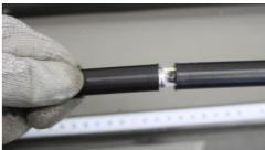
Pull the severed part off the middle sheath to get the yellow tear wires out.
