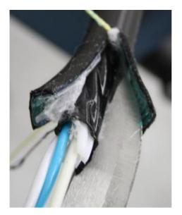
Scrape off the white ribbon under the armoring from one of the sheath halves and the plastic layer on the surface of the armoring.
