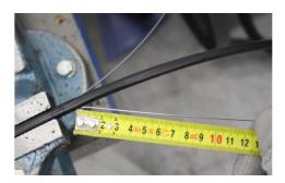
Cut the steel wires or fiberglass strength members to about 10 cm in length.
