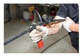
Peel the sheath off the steel wires, either for about 50 cm or for the entire length to be peeled.
