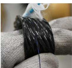
Bend the middle sheath away and find the black and blue tear wire on its inner surface. Remove the end of the tear wire from the sheath with the tip of the knife and pull the wire off the sheath to the split point.
