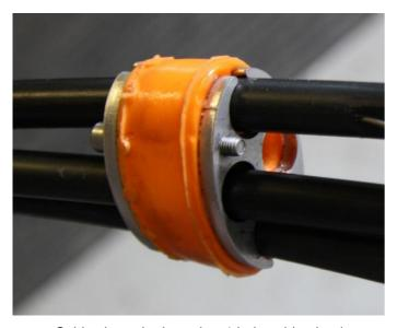
Cables brought through a 4-hole cable gland
