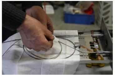
Place the paper used for cleaning on the splice tray to protect the tray from the grease of the fibers, as the grease inside the steel tubes is very tightly attached to the fibers.
