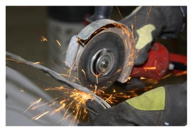
Cut the inner wires from the marked cutoff point, taking care of the steel fiber tubes in the middle of or between the wires.
