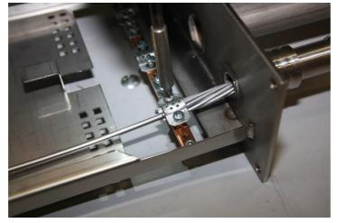
Insert the OPGWs into the joint closure and temporarily attach their inner wire layers to the grounding rail of the housing with corrugated arc fasteners.
