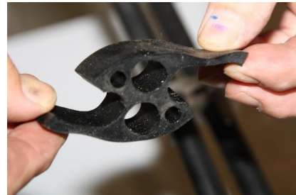
Split the pass-through holes used in the rubber part of the pass-through piece with a sharp thin knife.
