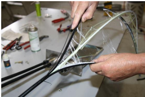
Cable splitting tool ST-OCS
