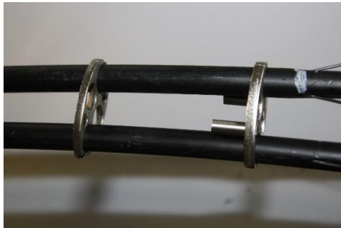
Pull the cable ends through the holes in the inner pass-through.
