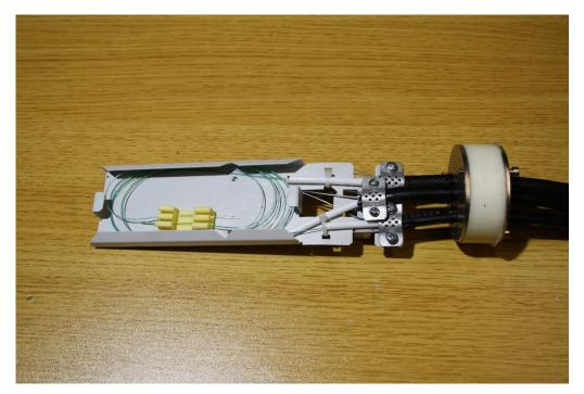
Place the fibers on the splice tray, cut off the excess lengths and splice the fibers.
