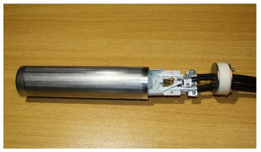
Push the inner part of the joint with the grommets inside the protective shell of the joint closure.
