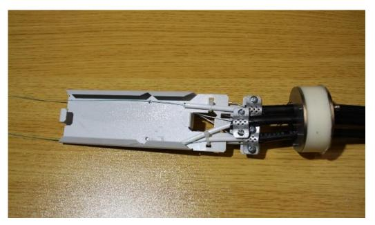
Mark the pealing points on the central tubes of the cables and cut the central tubes by making incisions around them with a cutting tool and bending the central tubes so that they come off. Pull the central tubes away from the fibers and clean the fibers from gel.
