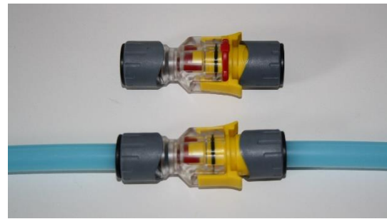
Gas-tight connector for 14/10 mm microducts. When choosing the connector, attention should be paid to the outer diameter of the microduct!
